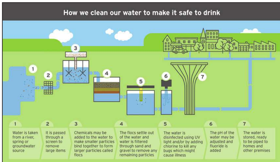
Treatment stages of piped water in cities
